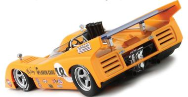
In comparison with the former 'M8', the M8D was wider and with a lower wing, which was also braced to the chassis, as the high mounted, suspension attached wings had been banned.
