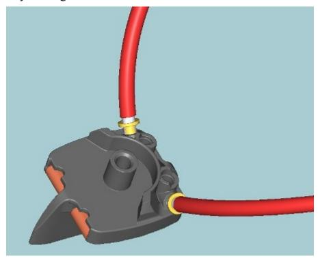
4. Secure braid and wire in place with the grub screws
