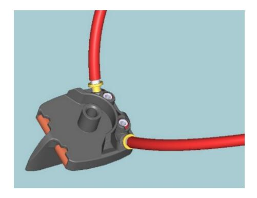
Pickup can now be secured in place with the provided washer and screw.
