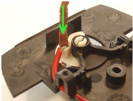
The braid must be thread in between the cable and the forward face of pick-up.
