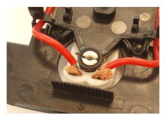
After completing the assembly, braids must be cut so that their ends don't pass the pick-up blade edge.
