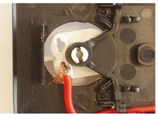
The assembly of cable and braid must be secured by putting an M2 grub screw 3 millimeter long. The screw must be inserted between the braid and the forward pick-up face.
