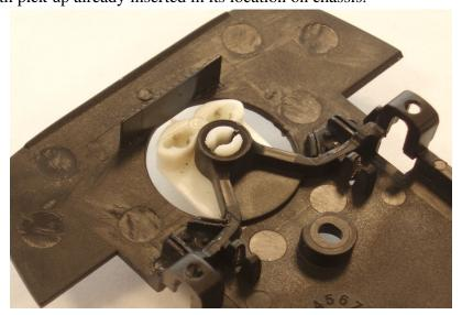
First, cable must be thread in its pick-up location, and then, the braid.
