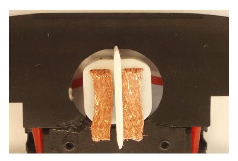
It's possible to put an M2 grub screw inside the pick-up shaft; the screw should be 6 millimeter long. This would make the pick-up more surely connected to chassis in the event of an impact; moreover, this allows to reduce the play of pick-up with its location.
